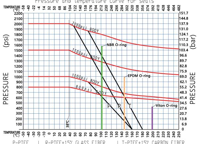
I R-PTFE+15% GLASS FIBER I T-PTFE+15% CARBON FIBER The data is only for your reference. The performance may be affected under different work situations.
